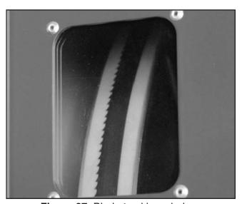
Figure 37. Blade tracking window.
